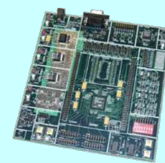
Virtex-II LC 1000 Memec Development Board
