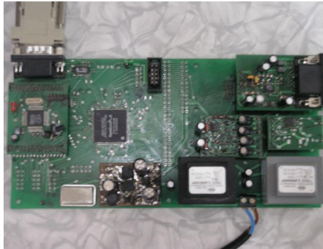
Fig. 4. Implemented hardware of the multichannel multipoint averaging circuit.
