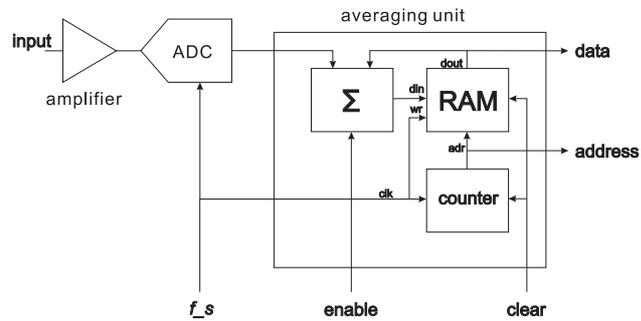
Fig. 1. A block diagram of a multipoint averaging circuit.
