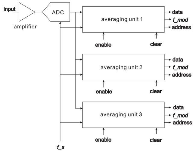
Fig. 3. A block diagram of a multichannel multipoint averager.
