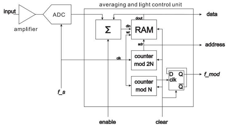
Fig. 2. A block diagram of a multipoint averaging circuit capable of producing synchronized modulation signal  $f_{mod}$ .
