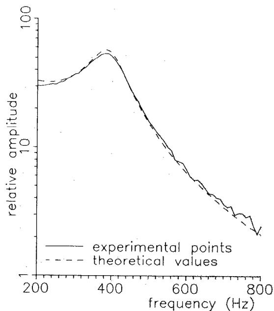
FIG. 3. Photoacoustic signal amplitude vs modulation frequency.
