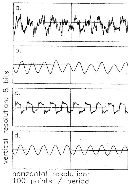
FIG. 2. Comparison of a typical photoacoustic response before and after digital signal processing. (a) Single trace of the recorded signal. (b) Strong noise reduction as a result of filtering. (c) Original shape of the signal obtained by averaging of 100 traces. (d) Nearly pure sine wave observed after filtering of the averaged signal.
