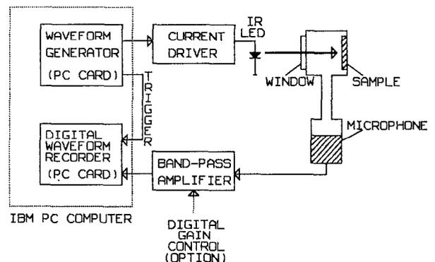
FIG. 1. Block diagram of an experimental arrangement for photoacoustic measurements. Structure of the system is based on concept of virtual instruments.
