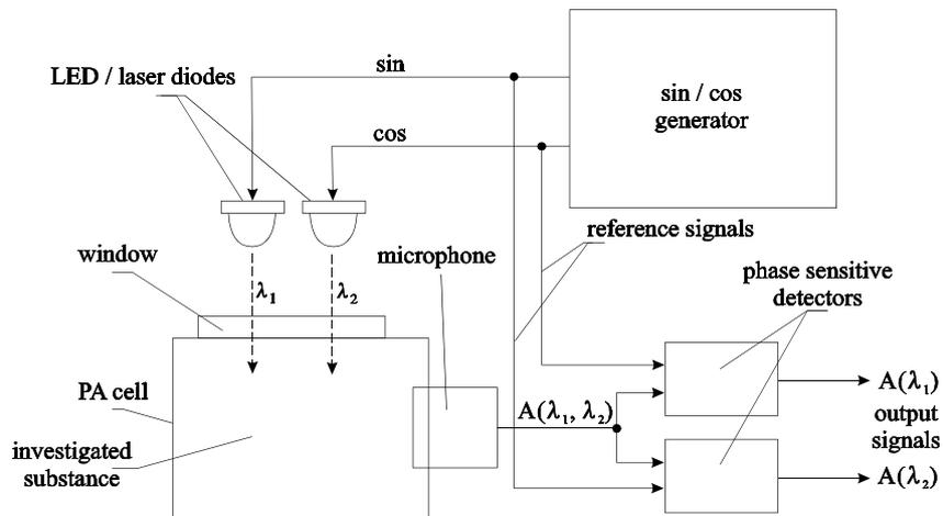
Fig. 1. Block diagram of a photoacoustic system based on orthogonal functions stimulation.
